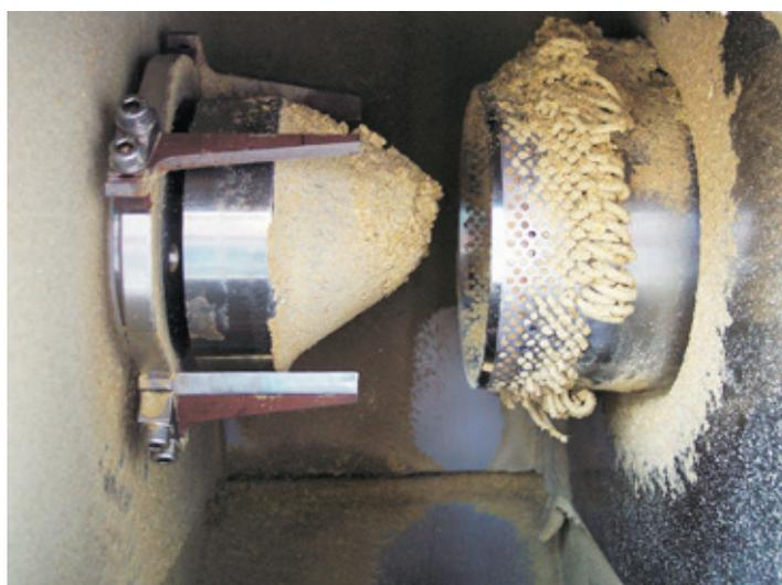
Fig. 3: Expander crown after shutdown
