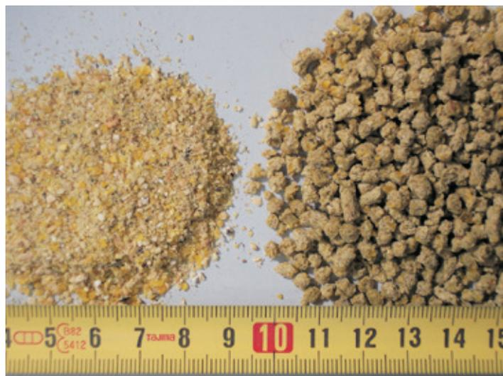
Fig. 4 Poultry feed before and after crown pelleting
