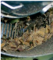
The wood chips are ground between pan grinder rollers and die
