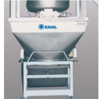
Proportioning weigher with 30 kg weighing capacity
