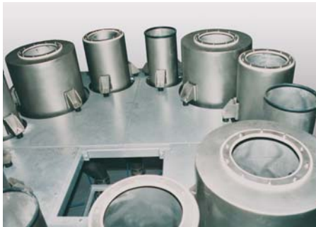
Component storage with 4 bins of 80 litres each, 4 bins of 160 litres each, and 4 bins of 360 litres each
