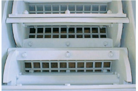
The particle size of the expanded product can be determined by means of the downstream crushing device.
