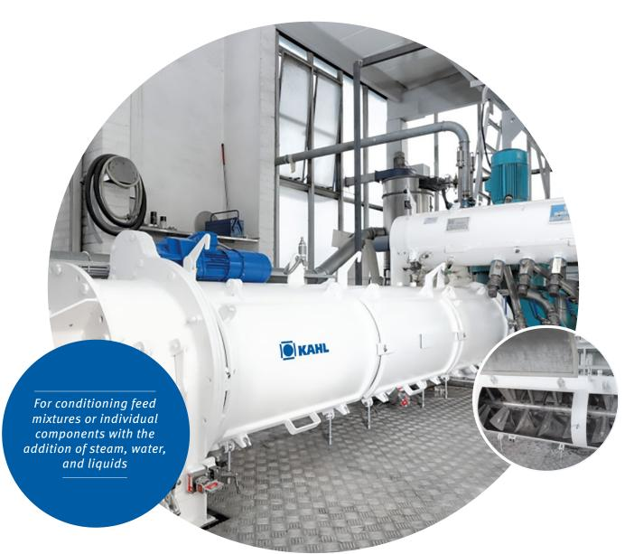
The optimum system for effective and economic thermal treatment of compound feed with firmly defined ratio of retention time and throughput. The MK is appropriate for the treatment of mash feed or as conditioner prior to the pelleting press.
