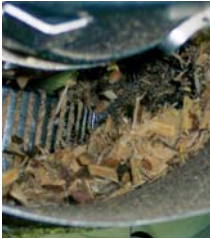
The wood chips are ground between pan grinder rollers and die
