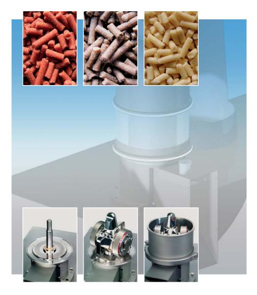
The granulation press is a high-performance laboratory machine with a very wide range of applications. The granulation presses have been designed for efficient dry granulation (agglomeration by compression) of food additives. The design of this series, which is especially appropriate for use in the pilot plant and as a small production machine, ensures an unmatched flexibility by using different pan grinder roller and die configurations as well as the positive drive of the pan grinder rollers.
