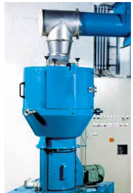
Caption: ROTOSPRAY®, type 700 (for high capacities)
