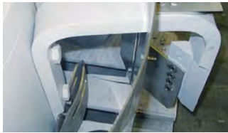
Pan grinder head with guide plates for the exact product distribution
