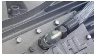
Gear oil spraying plant protects against overheating
