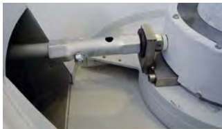
Pan grinder head stop for optimum adjustment of rollers and die
