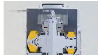
Hydraulic nut with quick-action coupling
