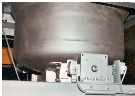
Weigh tank of the proportioning weigher
