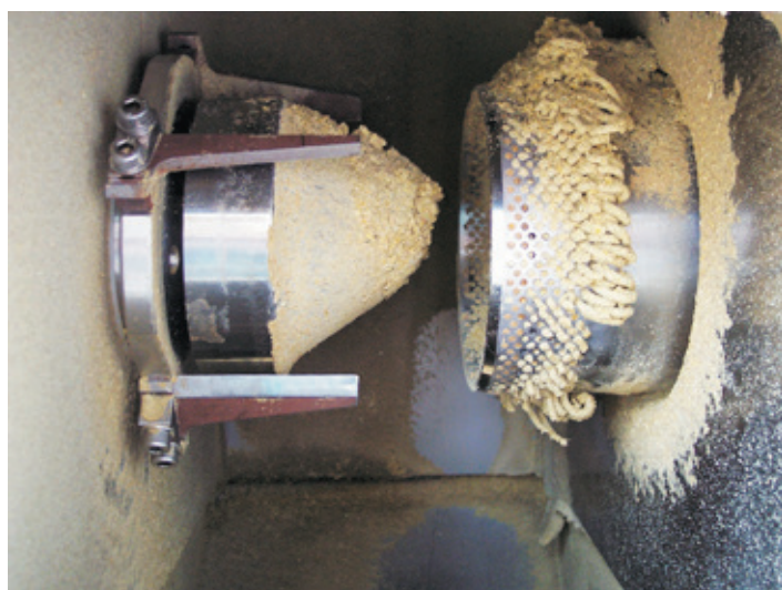
Fig. 3: Expander crown after shutdown
