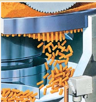
Cutting device for smooth edges and less fines.
