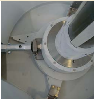
Pan grinder head stop for optimum adjustment of rollers and die.
