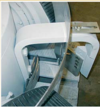
Pan grinder head with guide plates for exact product distribution.
