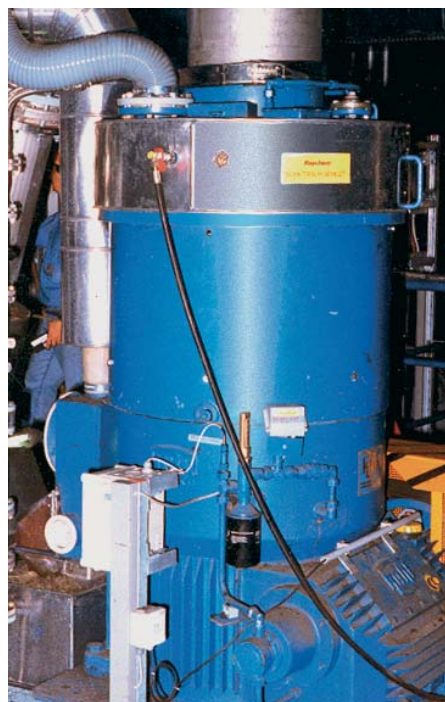
Pelleting press for the production of sewage sludge pellets
