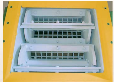
The particle size of the expanded product can be determined by means of the downstream crushing device.
